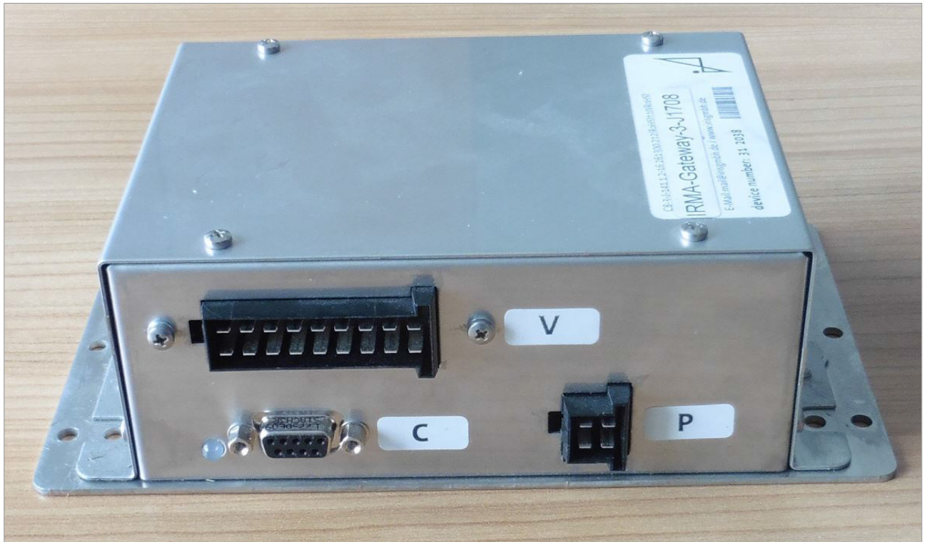
Fig. 2: View on IRMA-Gateway-3-J1708 operating interfaces and name plate
