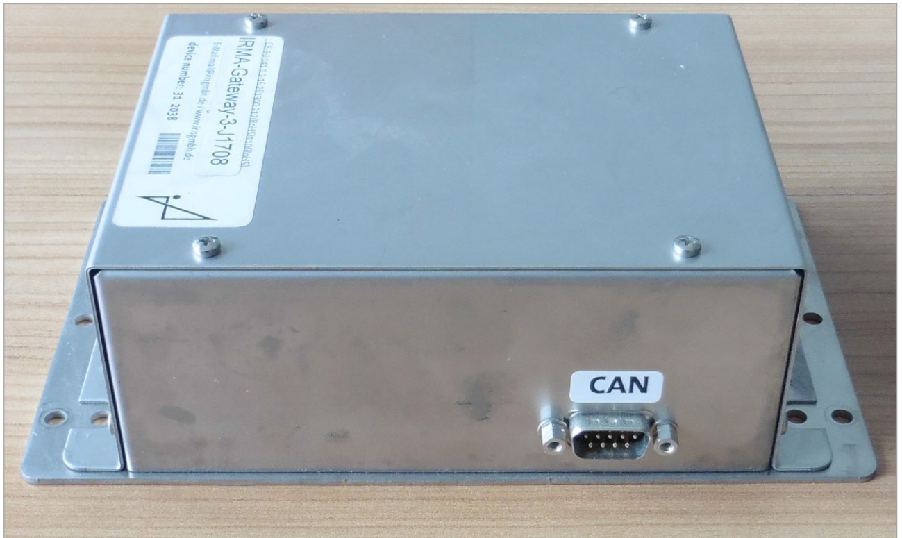
Fig. 3: View on IRMA-Gateway-3-J1708 CAN connector
